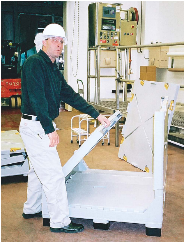
Wild Flavors' operations manager Peter Kindzierski demonstrates quick setup of the returnable bulk container, above, which arrives collapsed for easy shipment, below.
