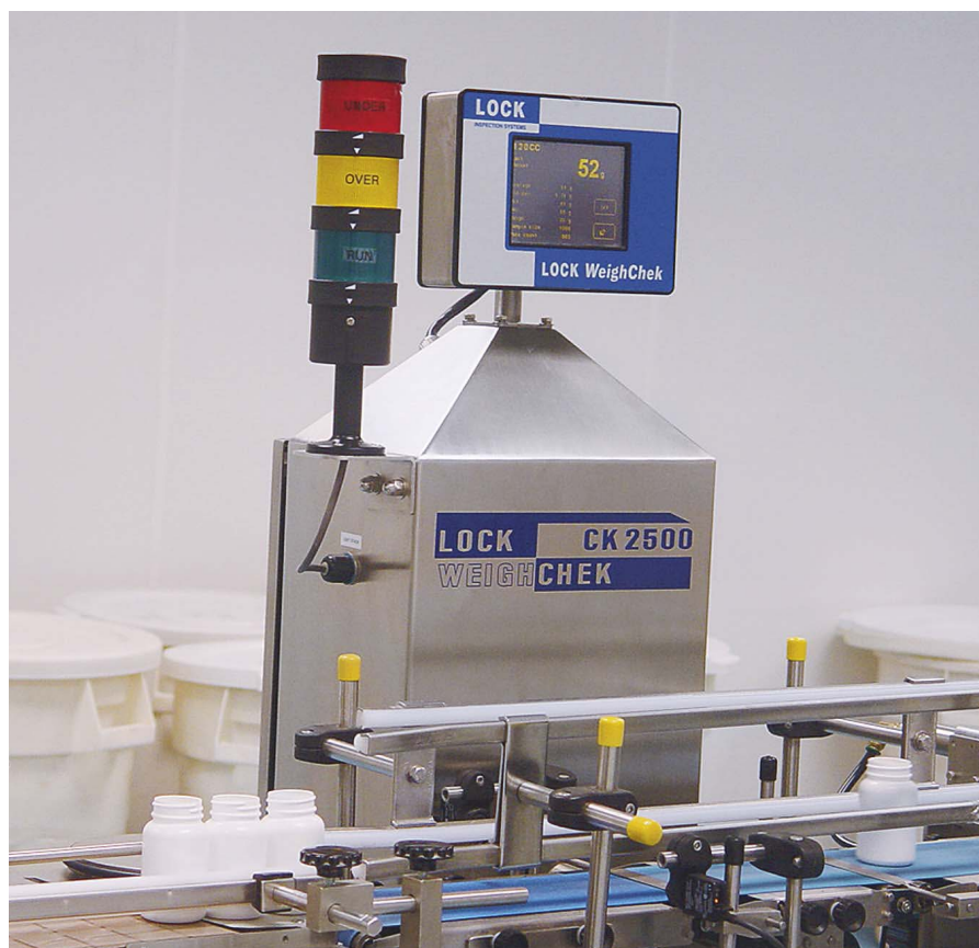
Recent plant expansions prompted West-ward to install more checkweighers and metal detectors. Bottles, above, move through checkweighers that are accurate to \pm 1 g.
