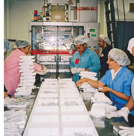
Operators hand-pick filled stick-packs of granular product as they exit the vf/f/s machine in groups of six.
